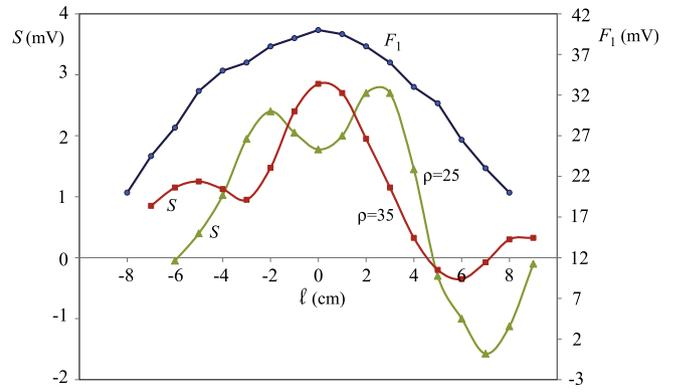
**Fig. 2.** Signal amplitude measured at fixed values of  $\rho$  (25 and 35 cm) as a function of the displacement  $l$  between the  $F_1$  launcher and the receiver. The upper curve, with its relative scale, represents the amplitude of  $F_1$  (once modulated and  $F_2$  halted) as measured for  $\rho = 30$  cm.
